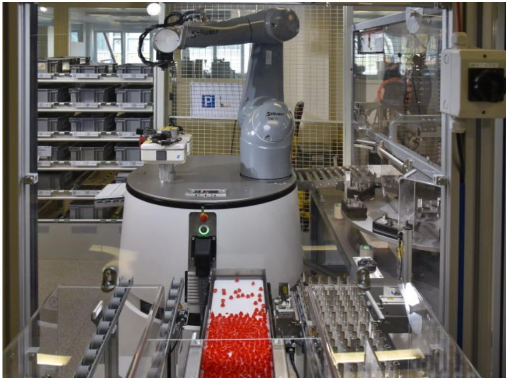
Figure 5.15: HelMo references itself at the workstation and starts loading the rotary table for the manufacturing of pneumatic couplings. ©Stäubli
