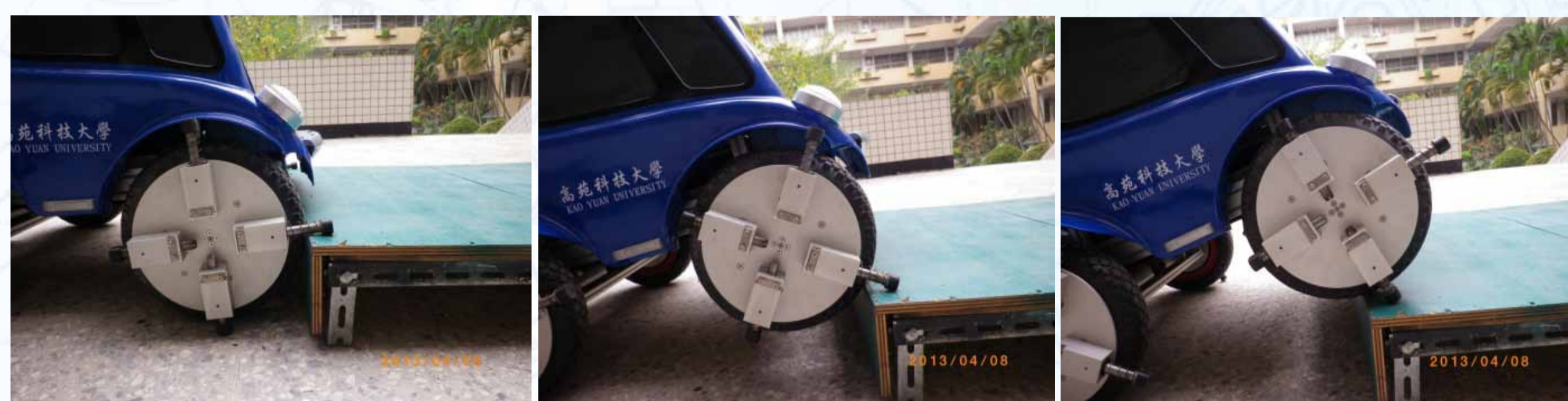
(a) 伸縮桿卡住階梯
