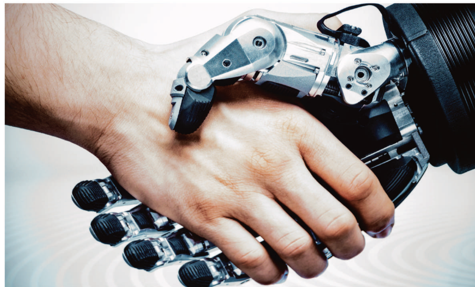
SCHUNK SVH 5-Finger Hand was the first robotic hand in the world to be DGUV-certified for collaborative use.
