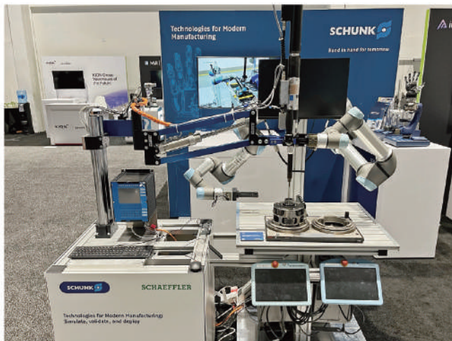
Developed in partnership: Automation exemplified by screw assembly application – digital and physical hand in hand.
