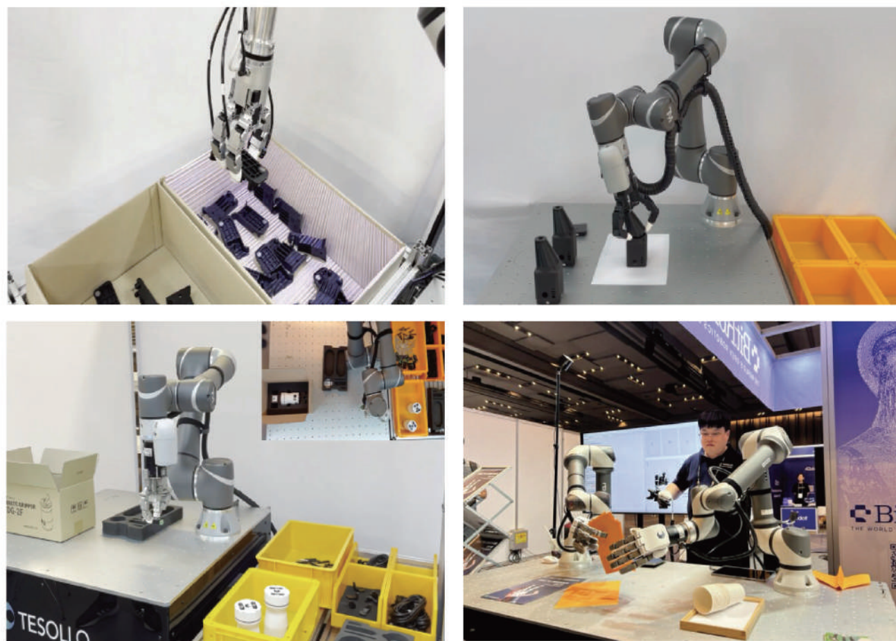
Figure 5. Various applications utilizing the DG-5F: bin-picking process (upper left), assembly process (upper right), re-alignment and packing process (lower left), and paper-folding task (lower right).
