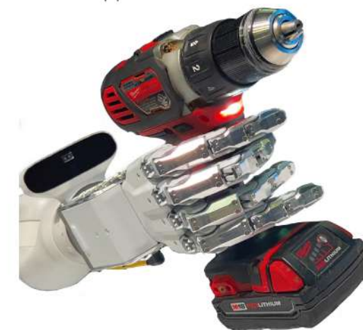
Figure 1. The ARTUS Lite's form factor and near-human capabilities allow it to handle complex shapes and conduct in-hand manipulation such as triggering a power drill, while holding the heavy and odd shaped object steady.
